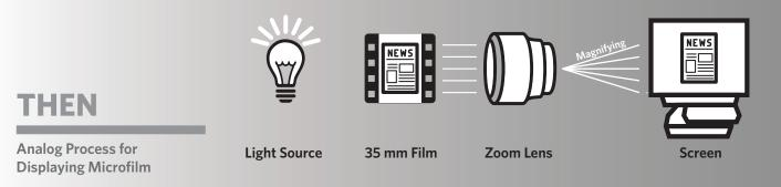
Typically, in the digital age of microfilm scanning, the lens most often is actually REDUCING not MAGNIFYING the object onto the miniature image sensor that processes, interprets, and creates the digital image which is then displayed on the monitor in real time. As can be seen, this makes discussing the benefits of Optical Zoom a largely outdated notion.
